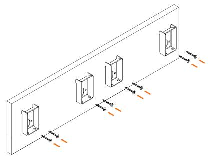
▶ Slide in alignment brackets halfway into the profile and tighten them using an allen key and provided headless screws.
